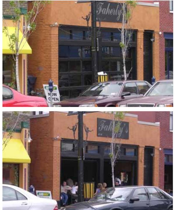
*Example of an operable window wall unit to provide open-air dining along street face.*
