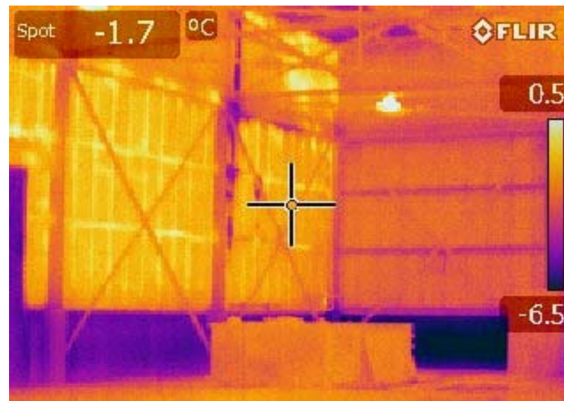
West Wall, North Corner, No Evidence of Infiltration
