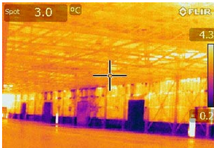
West Wall Thermal Imagery Readings, Evidence of Infiltration
