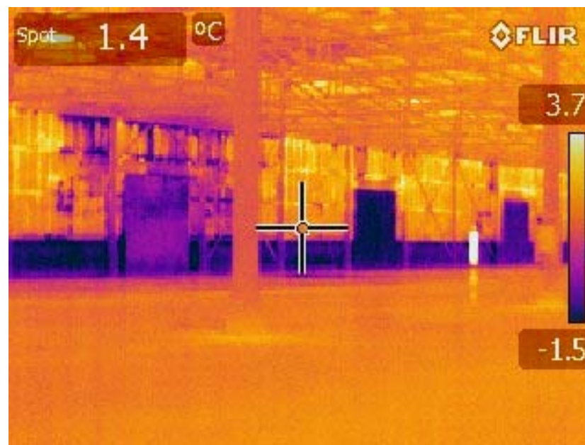
West Wall Thermal Imagery Readings, Evidence of Infiltration
